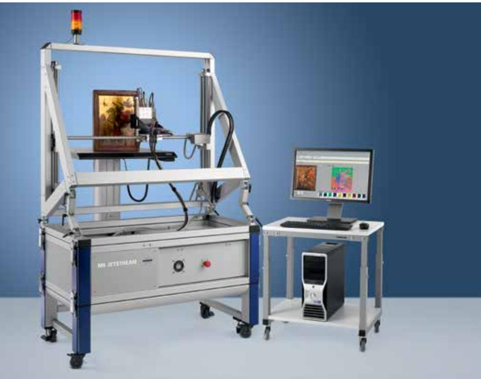
The Bruker M6 JETSTREAM is designed for the non-destructive elemental analysis of large samples. The mobility of the instrument allows it to be placed at the site of the object of interest, such as a gallery, museum or the shop floor. The performance parameters enable scanning areas of 800 mm x 600 mm with a variable spot size down to 100  $\mu\text{m}$  and speeds of up to 100 mm/s.
