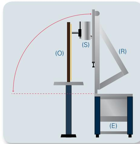
Diagram of the M6 JETSTREAM set-up in the upright measurement position, showing analysis object (O), spectrometer head (S), rig (R) and electronics compartment (E)
